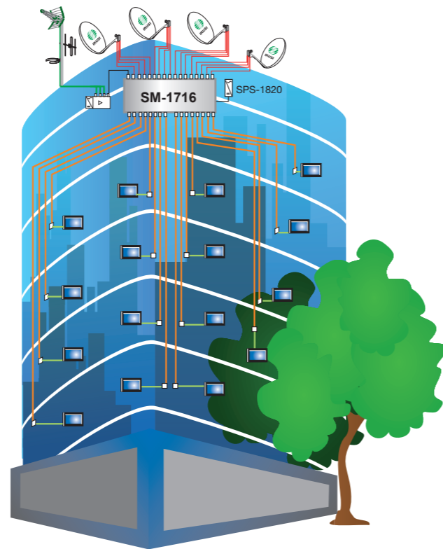
16 Sat-IF polarities plus Terrestrial through SM-1716 stand alone multiswitches
